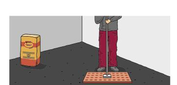
4. Compress and smooth the dry fill using a perforated wooden rammer. This fulfils two functions: the granulate chips are aligned horizontally and any air that remains in the insulating layer can escape. For fill heights of up to 80 mm, a single compression process is sufficient (if greater levelling heights are required, the fill is compressed once for approximately every
