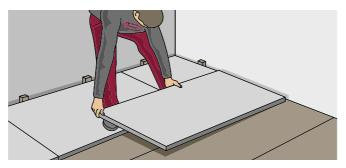
6. You can then immediately start with the floating installation of the base plates. Keep a distance of approx. 1.5 from the wall on all sides. To do so, fix wedges to the panels nearest the walls. These wedges must be removed again once the subfloor is completed.
