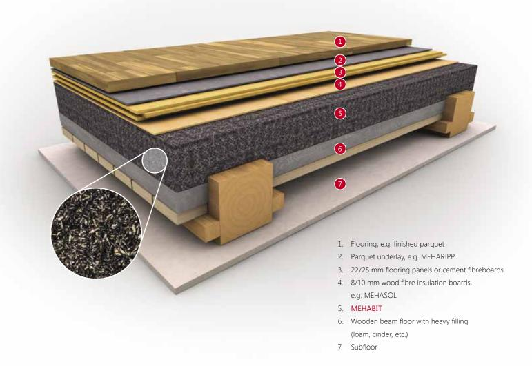
**MEHABIT** is a highly resilient, dust-free insulating and levelling fill as standard. It primarily consists of the ligneous stalk of the hemp plant, the so-called hemp hurd, which is impregnated using a solvent-free bitumen film that is also used for drinking water.
