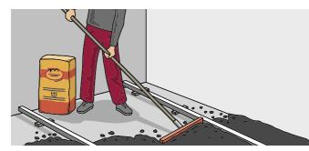
2. Spread the MEHA fills using a rake. It is possible that some of the MEHABIT has hardened slightly in the transport bags; however, you can easily crush these lumps.
